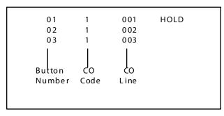
Buttons assigned as specific CO lines provide direct access and appearance of the CO line at a station. The station receives call status indications such as LED flash rates for incoming ringing when the line is placed on HOLD, etc. CO Line ringing is programmed in CO Line Attribute programming.
